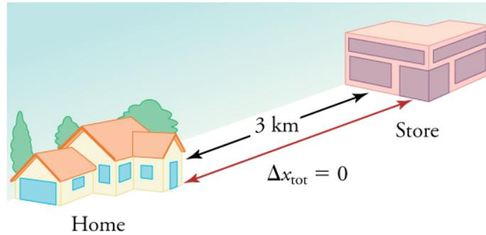
**Figure 2.10** During a 30-minute round trip to the store, the total distance traveled is 6 km. The average speed is 12 km/h. The displacement for the round trip is zero, since there was no net change in position. Thus the average velocity is zero.
