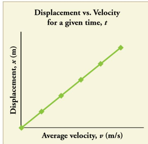
**Figure 2.27** There is a linear relationship between displacement and average velocity. For a given time  $t$ , an object moving twice as fast as another object will move twice as far as the other object.
