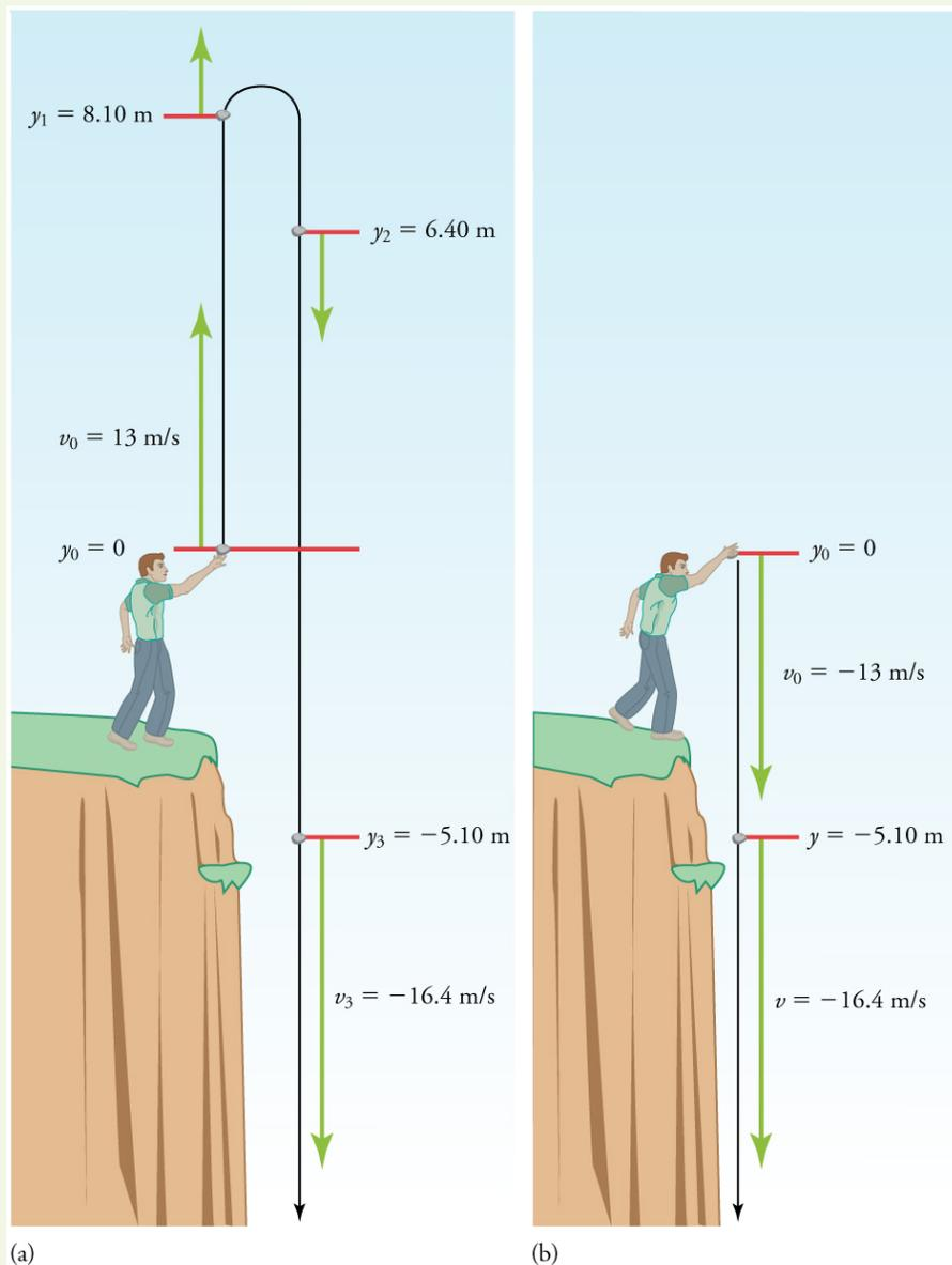
**Figure 2.42** (a) A person throws a rock straight up, as explored in [Example 2.14](#). The arrows are velocity vectors at 0, 1.00, 2.00, and 3.00 s. (b) A person throws a rock straight down from a cliff with the same initial speed as before, as in [Example 2.15](#). Note that at the same distance below the point of release, the rock has the same velocity in both cases.
