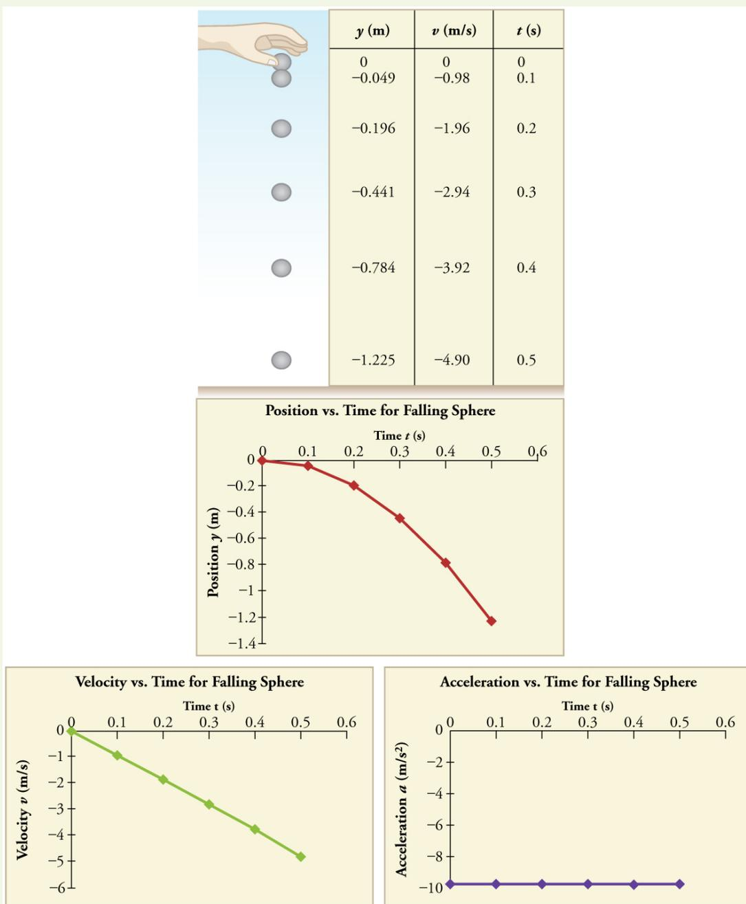
**Figure 2.43** Positions and velocities of a metal ball released from rest when air resistance is negligible. Velocity is seen to increase linearly with time while displacement increases with time squared. Acceleration is a constant and is equal to gravitational acceleration.
