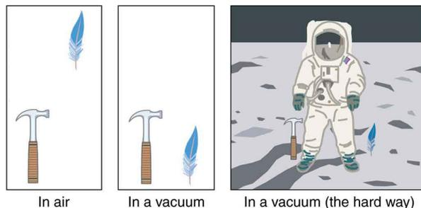
**Figure 2.38** A hammer and a feather will fall with the same constant acceleration if air resistance is considered negligible. This is a general characteristic of gravity not unique to Earth, as astronaut David R. Scott demonstrated on the Moon in 1971, where the acceleration due to gravity is only  $1.67 \text{ m/s}^2$ .
