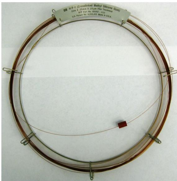
**Figure 4.3:** An example of a capillary column.
