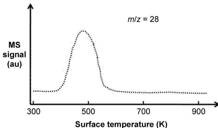
**Figure 4.15:** MS spectrum taken from a TPD experiment that CO ( $m/z = 28$ ) was first adsorbed on Pd(111) surface, followed by desorbing at a fixed heating rate. The desorption rate which is proportional to the MS signal reaches its maximum around 500 K.
