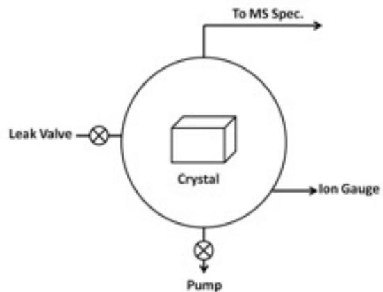
**Figure 4.13:** Schematic diagram of a TPD apparatus.
