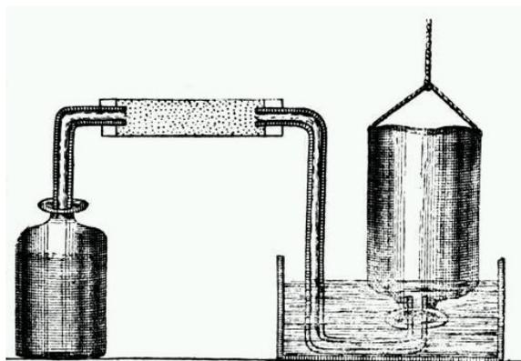
**Figure 2.8:** Cavendish's apparatus for making hydrogen in the left hand jar by the reaction of a strong acid with a metal and collecting the hydrogen gas above water in the right hand inverted jar.
